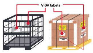
Label individual ULDs or pallets showing the gross weight of each unit that is to be collected for transport.
